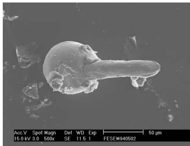
Fig. 7 Tensile fracture feature of the EFO wires. (Take 150 °C annealed wire for example)
